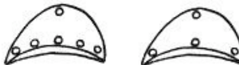
Figure 34 Motor Locations for 6 and 4 motor configurations
