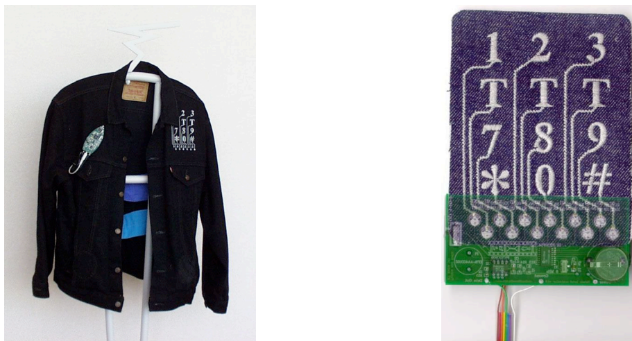
Figure 17 Keypad composite - denim E-broidered keypad and mating circuit board Image Credit: E. Rehmi Post / MIT Media Lab
